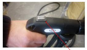
Chemical dosage is controlled via the pistol grip. Depress and hold the button on top of the pistol grip whilst simultaneously pressing the pistol grip
