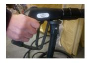
To operate the steam, pull and hold the trigger on the pistol grip.
