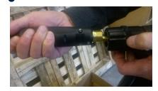
Select the required accessory and screw firmly onto the pistol grip in a clockwise direction. To change the accessory, simple unscrew in an anti clockwise direction
