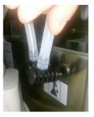
Firmly connect the chemical filler tubes from the chemical bottle to the rear of the machine
