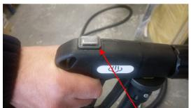
On the steam only hose chemical dosage is controlled via the pistol grip. Depress and hold the button on top of the pistol grip whilst simultaneously pressing the
