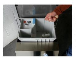
Remove the waste tank and empty.
