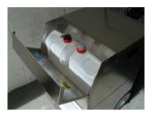
Fully open front cover, fill water tank with clean cold water. If required, fill chemical tank with manufacturers approved detergent. Replace cover.
