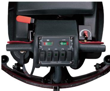
Easy-to-use operator panel with battery level indicator
