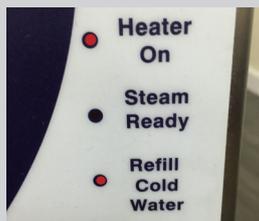
17. Refill Cold water when the refill cold water light illuminates and a intermittent beeping noise can also be heard.
