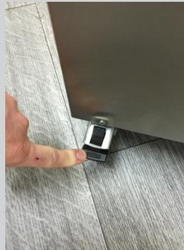
8. Push your machine to a suitable area and lock the brake lever to avoid the machine moving during use.
