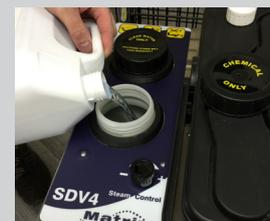
18. If detergent stops working. Refill detergent tank with suitable detergent.
