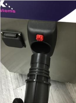
6. Connect vacuum hose, clicking it into position. Ensure it cannot be pulled out.
