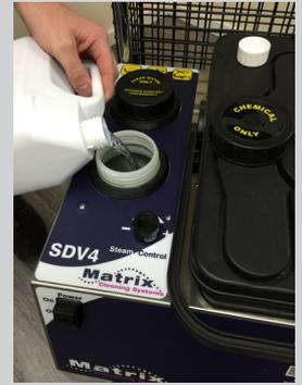
5. If desired. Fill the detergent tank with suitable detergent.
