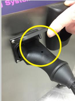
7. Lift the flap and connect the hose ensuring the pin locks into position.
