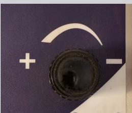
15. The steam output can be adjusted by turning the steam control.
