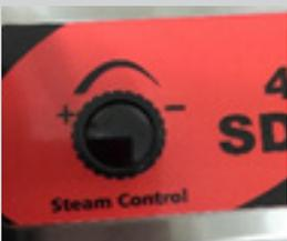
**15.** The steam output can be adjusted by turning the steam control.
