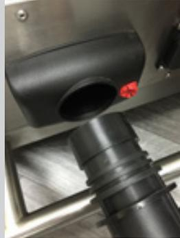
**7.** Connect vacuum hose, clicking it into position. Ensure it cannot be pulled out.
