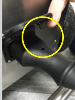
**8.** Lift the flap and connect the hose ensuring the pin locks into position.
