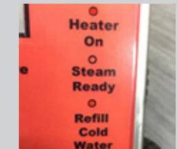
**17.** Refill Cold water when the refill cold water light illuminates and a intermittent beeping noise can also be heard.
