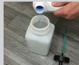
**18.** If detergent stops working. Refill detergent bottle with suitable detergent.
