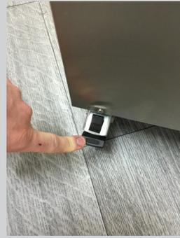
3. Push your machine to a suitable area and lock the brake lever to avoid the machine moving during use.
