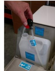
Remove Red water reservoir cap and fill with clean cold tap water. Fill 2nd reservoir if required and close lid
