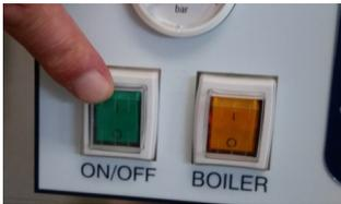
Plug machine into a suitable electric socket and press top section of green on/off switch
