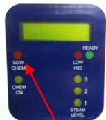
This light, when illuminated, indicates the chemical tank needs refilling
