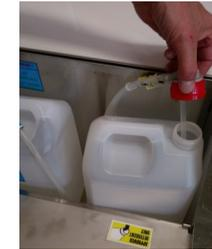
Open chemical container compartment at the rear and fill with manufacturers approved chemical if required
