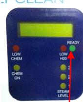
Allow 9 mins for the machine to heat up. The machine is ready when the Green Indicator light illuminates
